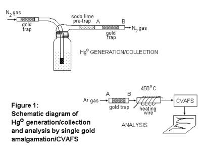
• Section 6.4.3 specifies the use of acid fume pretraps consisting of 8-14 mesh soda lime chunks and which are purged with nitrogen. For the manual system, BAL uses pretraps consisting of the sector of the chunks and which are purged for the with nitrogen.
