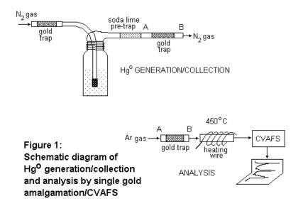
• Section 6.4.3 specifies the use of acid fume pretraps consisting of 8-14 mesh soda lime chunks and which are purged for 1 hour with nitrogen. BAL uses pretraps consisting soda lime chunks and which are purged with nitrogen.
