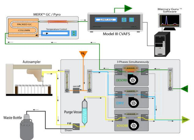
Figure 1. Diagram of sample flow path and connections for MERX MeHg analytical system.
