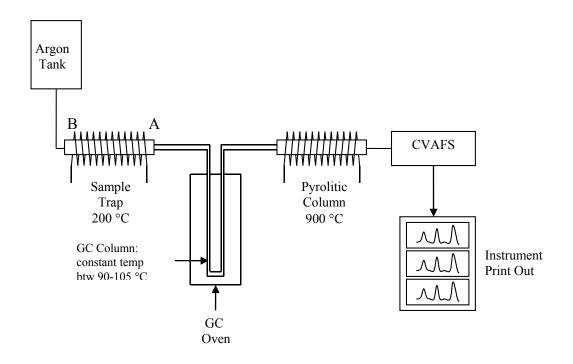
Figure 2: A schematic diagram of the isothermal Gas chromatograph system
